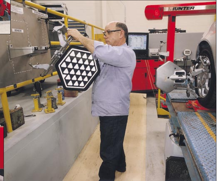
Proving Grounds staff designed this unique Hunter DSP400 Sensor target storage apparatus to meet their specialized alignment and audit requirements.
