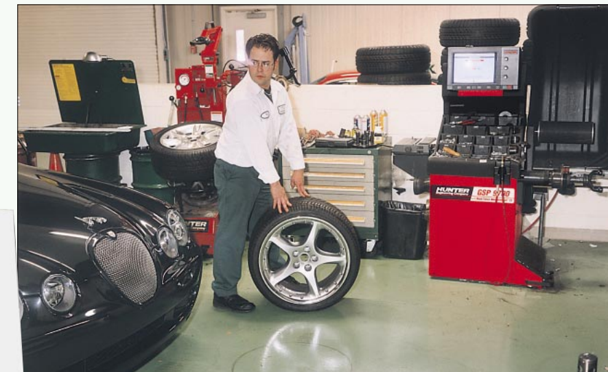
Technicians at Jaguar's U.S. Headquarters Technical Center in New Jersey use the GSP9700 to isolate wheel vibration. Jaguar, an early advocate of GSP9700 technology, recently named it minimum required equipment for dealer service.
