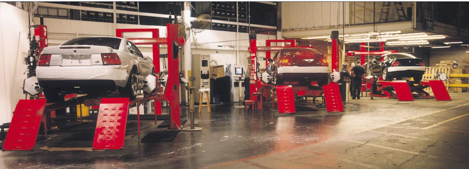
Hunter Series 611 Alignment Systems audit high-speed assembly alignment and serve as a benchmark at Ford's Dearborn production facility.
