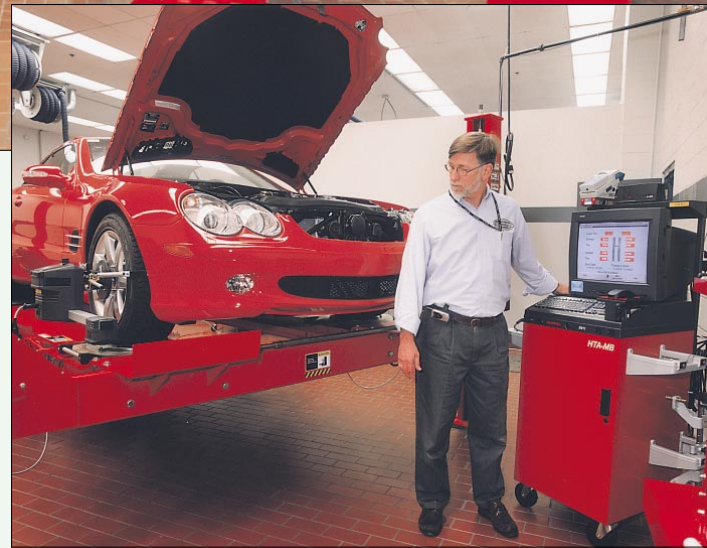
Mercedes-Benz USA technical staff use two Hunter HTA-MB alignment systems at the carmaker's headquarters in Montvale, New Jersey. The systems include Hunter 12,000-lb. capacity 4-post MKS alignment racks with extended runways that easily accommodate top-end Mercedes-Benz vehicles including the new Maybach.
