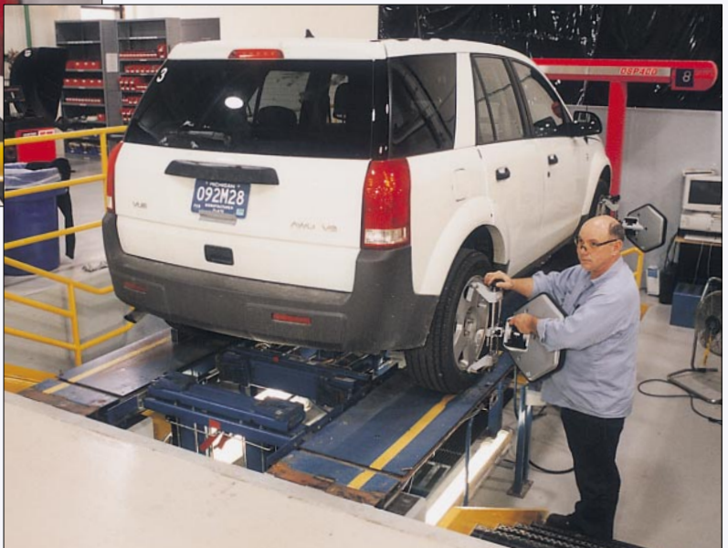
Designated "North" and "South" Pit Racks, these Hunter alignment systems serve the entire Milford vehicle engineering operation.
