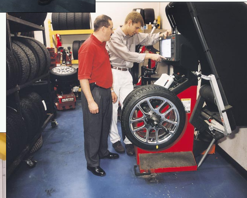
Hunter Sales Representative William Keyes and a Viper Engineering staff member measure the radial force variation of a high-performance Viper wheel assembly.
