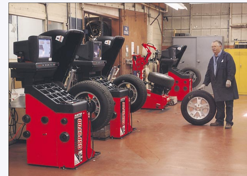
The Tire Uniformity Grader or "TUG", visible behind the glass partition, now shares lab space with the same Hunter GSP9700 Vibration Control Systems that are available to Ford dealership service departments.
