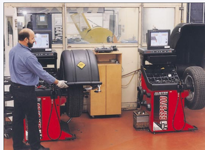
The Tire Uniformity Grader or "TUG", visible behind the glass partition, now shares lab space with the same Hunter GSP9700 Vibration Control Systems that are available to Ford dealership service departments.
