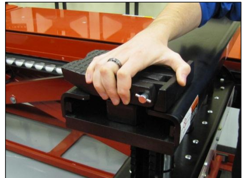
Ensure that the lifting pads are retracted before completely lowering jack.
