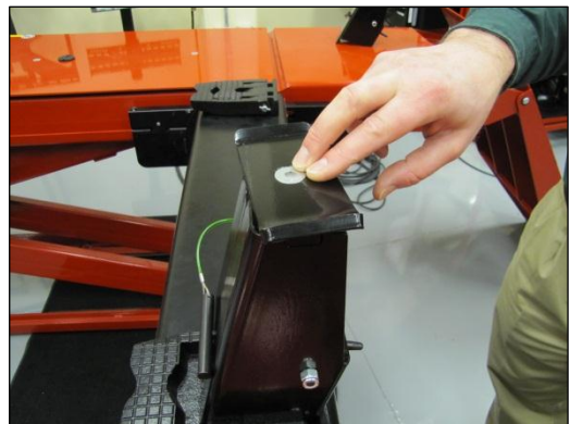
Correcting lifting location.
