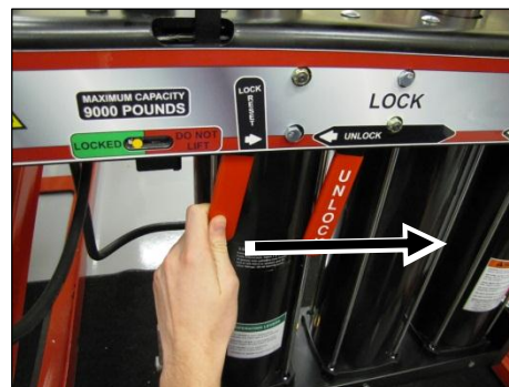
Move the reset lever to the right to re-engage the locks.
