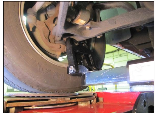
Correct lifting location.
