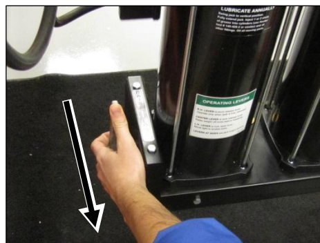
Lower the upper beam onto the locks.
