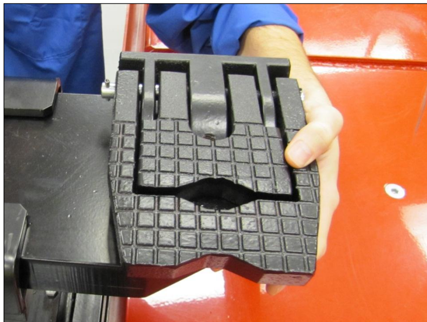
Lifting pad shown in the fully collapsed position.
