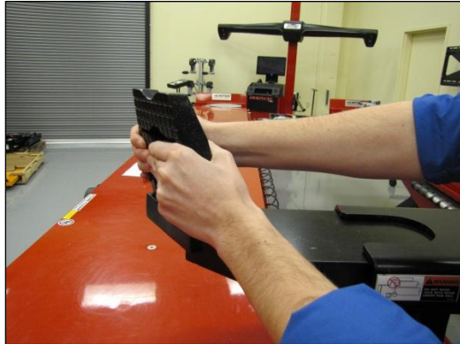
To stow lifting pad, pull up to disengage the lock.
