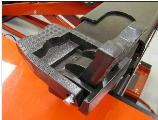
Smaller, inner lifting pad raised.
