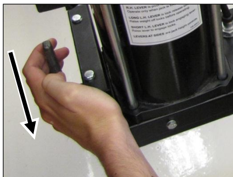
Lower the jack to just above the desired height.
