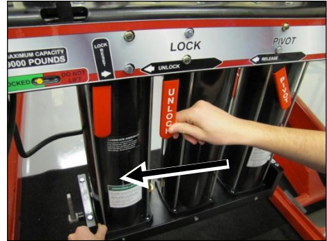
Move the lock release lever to the left.
