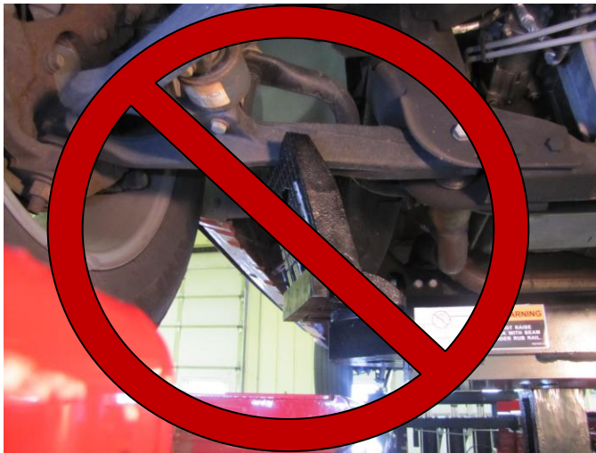
Incorrect lifting location.
